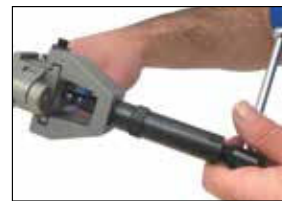
Step 4 Turn T-Bar to create the flare
