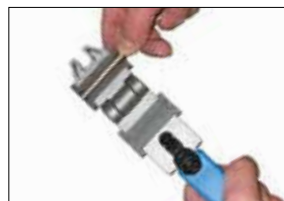
Step 1 Place the pipe in the die
