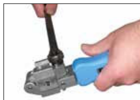
Step 2 Tighten the clamping nut
