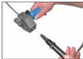
Step 3 Insert the punch and ram
