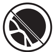
DO NOT USE A DAMAGED WHEEL
