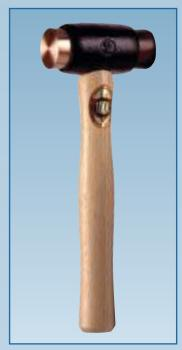
Cast-iron head fitted with one face of pure electrolytic copper, the other of compressed water buffalo hide and fitted with wood handle.
