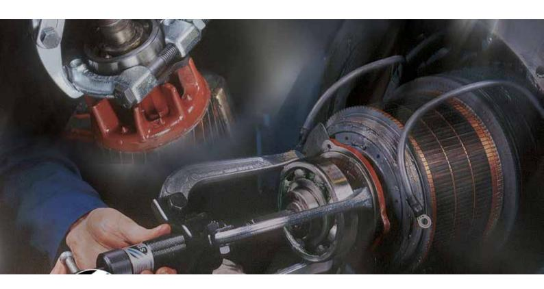
Sykes-Pickavant pullers are manufactured to a very high specification and subjected to rigorous testing - far exceeding their stated capacities. The legs and beams are drop forged from high quality steel and then heat treated for extra strength and durability. Pullers are normally classified as either hydraulic or mechanical with many different types within these two styles.
