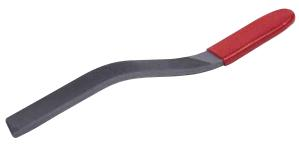
**Bumping Tools** - these are used for slapping out dents, with or without the backing support of a dolly. (For slight dents or a wavy surface, a dolly is not required). They should only be used where damage is moderate or slight, they are not intended to take the role of the spoon or beater and dolly.
