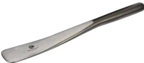
**Spoons** - spoons are used for bumping and prying, they can also be used instead of a dolly when direct access to the rear of a panel is obstructed. The choice of spoon depends on the original contour of the metal, the amount of access available and the proposed action (ie roughing or levelling).
